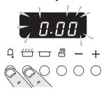
Press and hold as above. At the same time, press (-) or (+) until the correct time shows. Don't forget it's a 24 hour clock. If you make a mistake or press the wrong button, turn off the power supply for a minute or two and start again.
